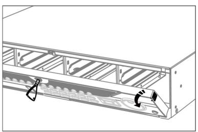
Figure 1-6 Open Front Panel
