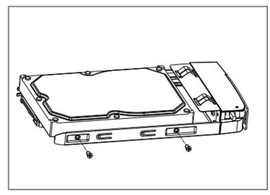
Figure 1-8 Fix HDD
