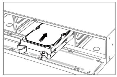
Figure 1-7 Insert HDD
