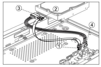
Figure 1-11 Connect Cables
