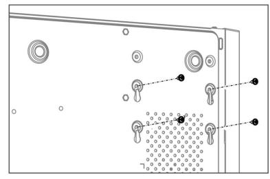
Figure 1-12 Fix HDD to Device Bottom
