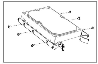
Figure 1-5 Fix Mounting Ears to HDD
